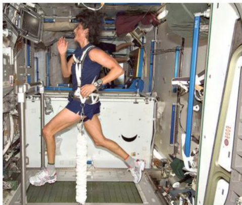
Astronaut Sunita Williams uses the treadmill onboard the ISS in 2012. The harness is visible reaching from the treadmill's base to a ring on her hip. NASA
