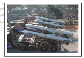
The Brahmaputra River in India and the Moskva River in Russia are the sources of the name. It is a two-stage missile with a liquid-fuelled ramjet engine and a solid-propellant booster. It can achieve Mach 3.
