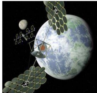
A conceptual illustration of a satellite collecting solar energy in earth orbit and beaming it down as microwaves. NASA
