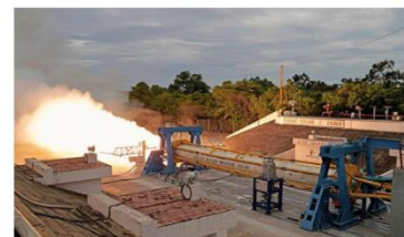
The ground test of the SOLVE solid motor being conducted at the Satish Dhawan Space Centre in Sriharikota. SPECIAL ARRANGEMENT
